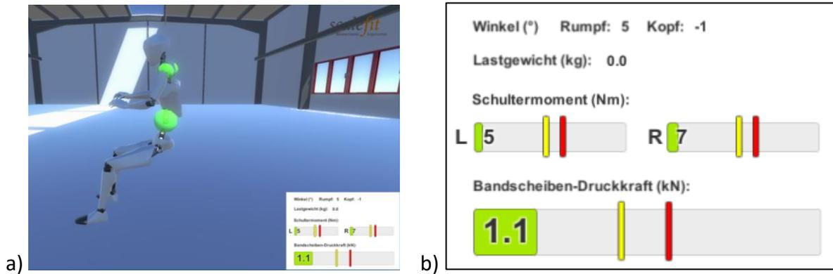
Fig. 3: a) Evaluation monitor and b) evaluation routine (enlarged) in Unity-3D
